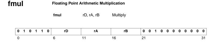
The floating point value in rA is multiplied with the floating point value in rB and the result is placed into register rD.
